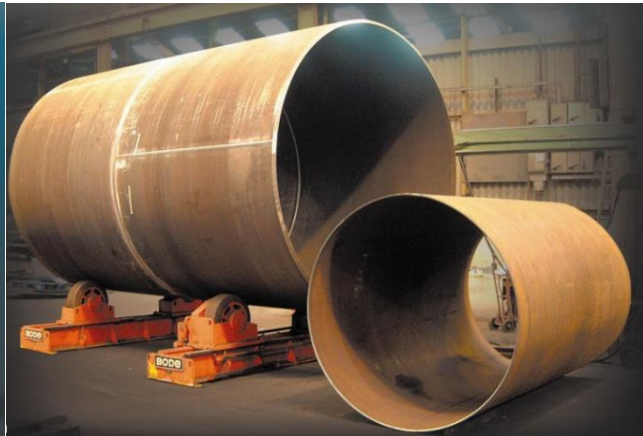
2m pipe segments welded together(big diameter)
