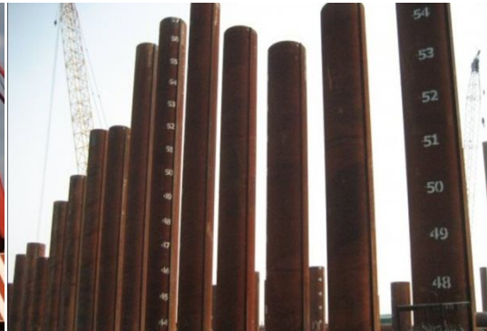
Van Phong Terminal Project phase II Vietnam 800x18, Length minimum 55meters
