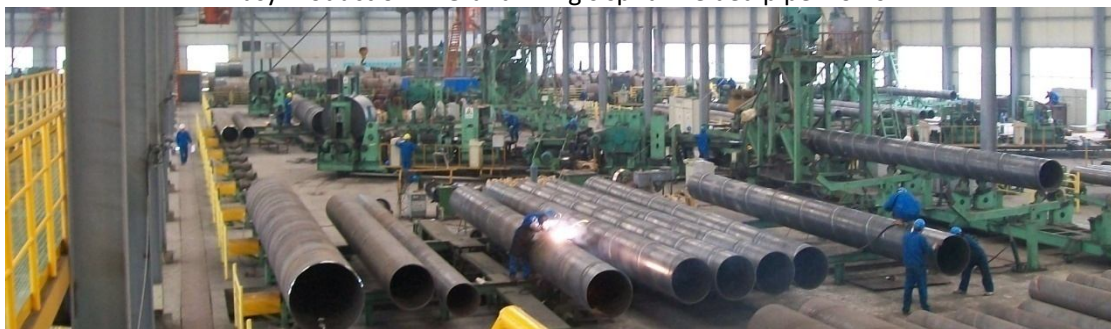
Busy Production in Grand Piling's spiral welded pipe works
